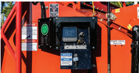
Infeed-Mounted Control Panel
